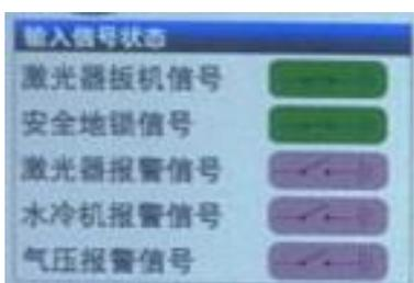
Figure 3.3.6 Monitoring Page - Input Signal Status Bar
