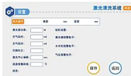
First click "Settings", in the pop-up window of the password input page to enter the password 123456, you can enter the settings page, cleaning mode settings page compared to the welding mode deleted some of the parameters not useful for cleaning, adding the "gun head model" and The setting page of cleaning mode has deleted some parameters that are not used for cleaning, and added "head model" and "trigger setting" two parameters that are dedicated to cleaning.
