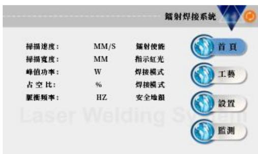
① This interface allows you to see the current process parameters (process cannot be modified on this page) and real-time alarm information.
