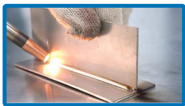
Internal fillet welding
