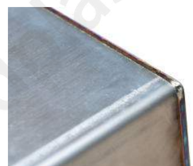
Outer Corner Welding
