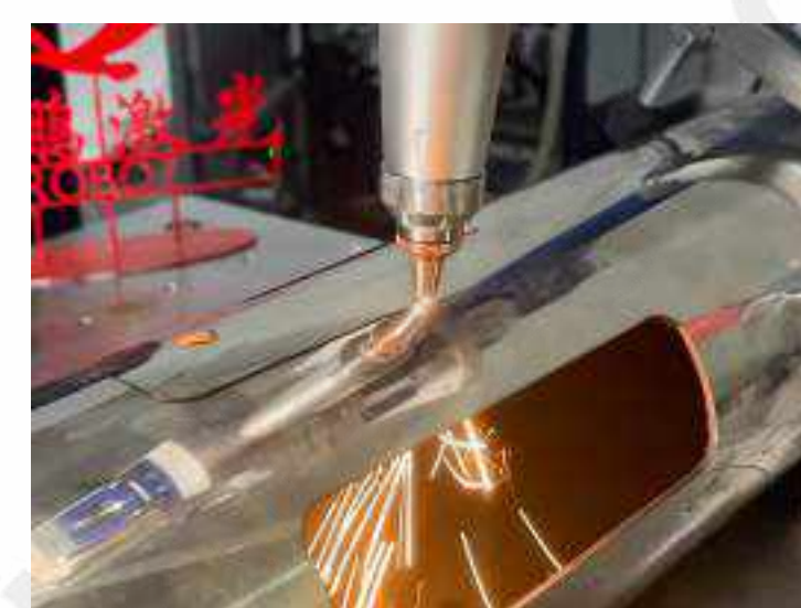
3D Cutting of Pipes
