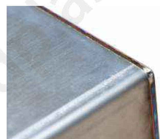
Outer Corner Welding
